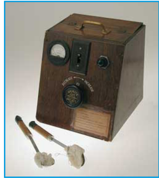
Figure 2: Kouwenhoven's open chest defibrillator [10]
